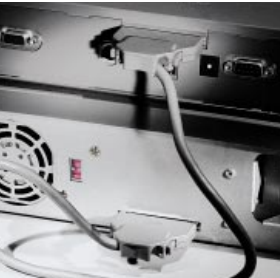
The Port Replicator connects with the Expansion Station for maximum flexibility.
