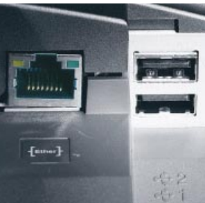
The Equium 2000 ships with an Ethernet adapter for network connectivity and two hot plug-and-play USB ports.
